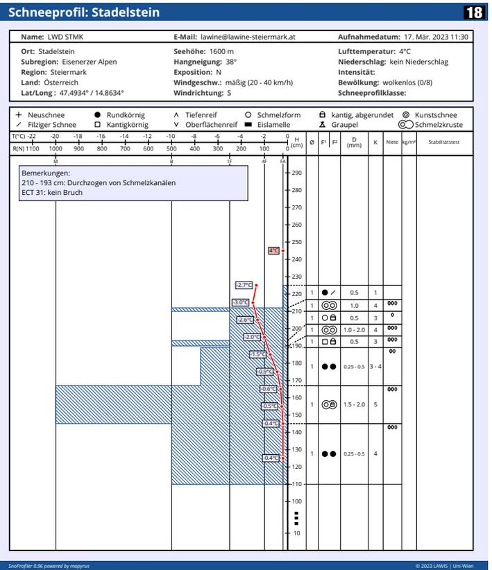
Small text at the bottom of the snow profile chart: "SnowProfilier 0.36 powered by mesyris" and "© 2023 LWDWS | Leo-Wein"
